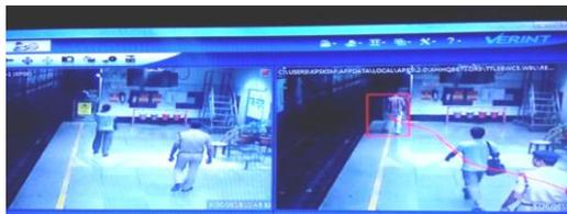
An intelligent video analytic software has been programmed and installed at Park Street station and put on operation. Such system can detect unidentified luggage, increased passenger density, passengers crossing yellow demarcation lines at platform, etc. and provide audio-visual alarm at the SM's office as well as Central Security Control. This arrangement has made Metro stations more safe & secure to the passengers.
